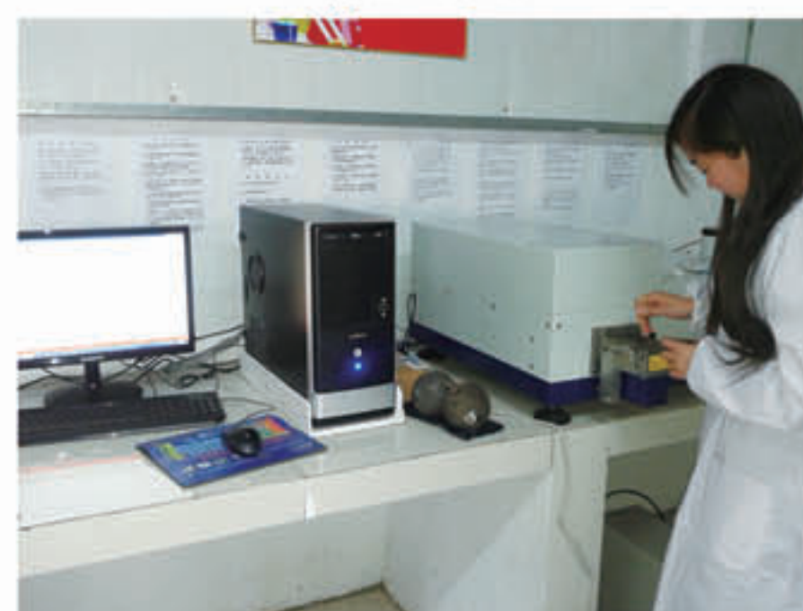
光谱仪用于检测化学成份 Spectrometer Is Used To Detect Chemical Composition
