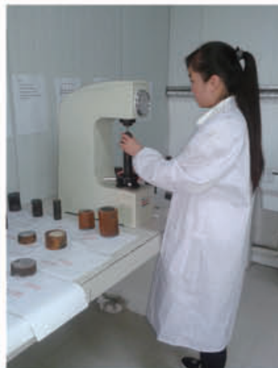
洛氏硬度计 Test Instrument For Hardness
